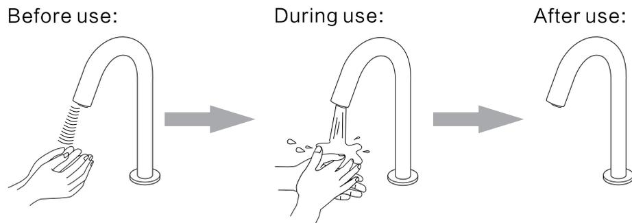
Note: when your hand enters the inductive field the water flows, remove your hand from the field and the water stops. It will stop automatically after flushing 30 seconds continuously, leave your hand from the inductive field for 3 seconds then enter the field to flush again.
