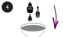
Remove any O-rings and soak all components in de-scaler. Rinse throroughly in clean water. Examine all seals and replace if needed. Use a WRAS approved silicon based grease on all seals.
