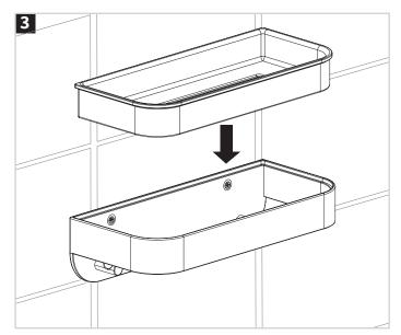
Place the basket insert on the metal frame and push down until you hear a "click". The basket can be removed for regular cleaning and maintenance.
