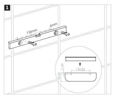
Remove the basket insert and mark the location of the holes on the wall, ensuring the holes are not on the edges of a tile or on the tile grout.
