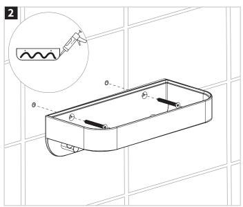
Fix the basket to the wall using the screws provided. Apply a bead of silicone sealant to the back of the basket to make watertight. Check the manufacturer's instructions for drying times
