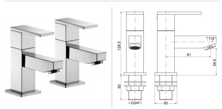
Dimensions are in millimetres except thread sizes which are BSP imperial.
