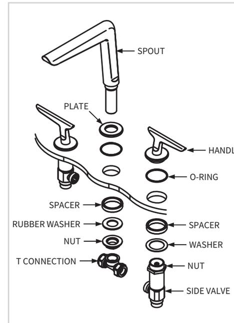
Fix the side valves to the basin, securing with the handle assemblies from the top and the spacers (if necessary), washers and backnuts from the bottom. Confirm that water exits on side valves are pointing to the center. Handles should be pointing outwards when closed and towards you when open.
