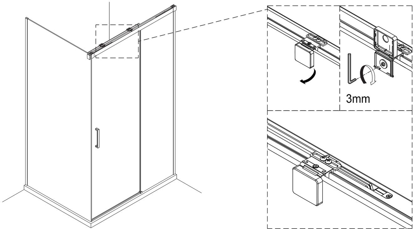
Step 16-2: Loosen the screws at both ends of the roller track slightly.
