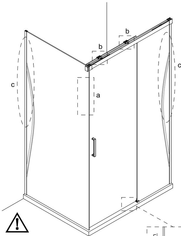
Adjust the sliding door using the middle screw located on top of the roller. Loosening the screw will move the door upward and tightening the screw will move the door downward, please ensure there is a 7-9mm gap between the bottom of the sliding door and the shower tray.
