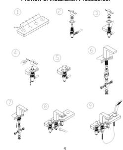
Installation Procedures: Step 1:Drill four holes on the bath as per the drawing shown below.
