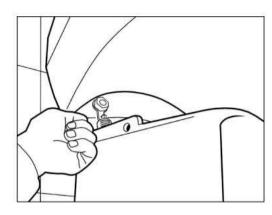
4. At the same time the semi-pedestal is placed under the washbasin. The hook of the spring stretched to the fixture hole of the semi-pedestal is attached to the hole.
