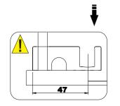
Please note that the width of the sliding guide which stands on the tray threshold should be no less than 47mm.
