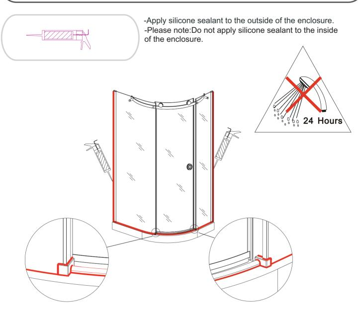
Silicone(according to the thick line position) where the vertical profiles meet the wall, parts meet parts and the glass panels meet the tray.
