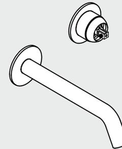
6. Fix the valve to the supporting framework using the screws provided.
