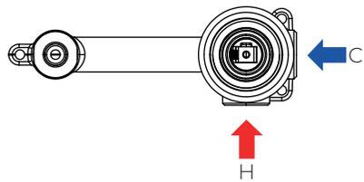
1. Ensure the pipework is correctly arranged to suit the position of the hot / cold inlets (etched on the valve body).
