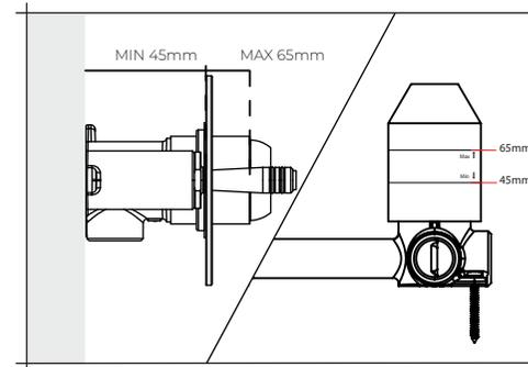
3. Ensure the valve is set back from the finished front face of the wall by the correct depth of min 45mm max 65mm (Allow for tiles, adhesive, etc).
