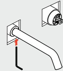
5. Ensure the pipework is correctly arranged to suit the position of the hot / cold inlets (etched on the valve body).
