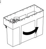
Tank can be rotated for left or right bottom inlet. NOTE: Connection position is diagonally opposite when reversed. If not accessible, plumb connection before mounting the cistern. Please do NOT leave the knock outs in the tank once popped out.
