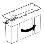
Side inlet is located on the left side of the tank. However, the tank is reversible if right hand inlet installation is required.
