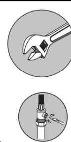
Connect the hot and cold water connections.
