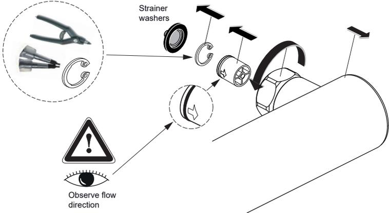
3. The check valves are housed inside the retaining inserts within the inlet bores. Look closely at the rear of the mixer body.
