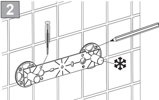
Place the brackets over the exposed pipes and use the template provided to position them 150mm apart.
