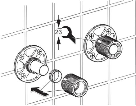
Slide the olives onto the pipes. Screw the two connectors onto the wall brackets by hand until they stop against the olives.
