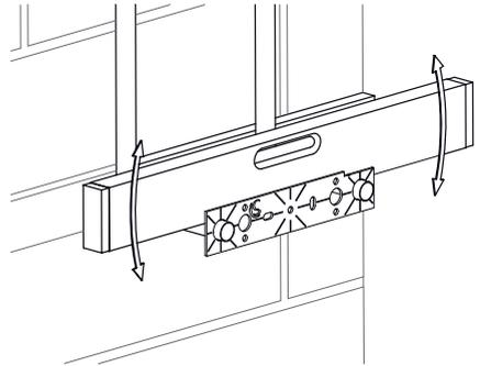
Ø15mm copper supply pipes should be run within the wall cavity.
