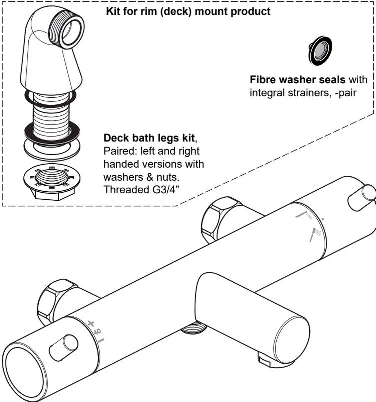
Deck bath/shower mixer shown without deck mounting legs assembled. Supplied with only **A7593AA** product. Right side handle controls flow & diverts between bath fill & shower hand set.
