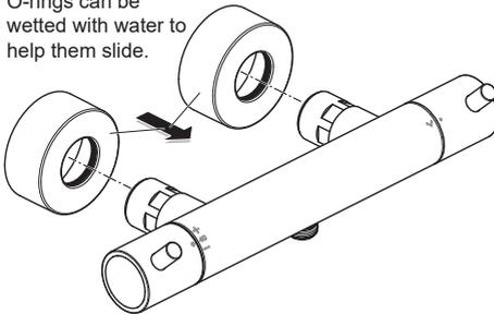
When the sealant has set, slide the covers onto the inlet legs (captive nuts) of the mixer. The covers have o-rings fitted in the bore, ensure the flats on the captive nut remain exposed to allow them to be screwed onto the adaptors.
