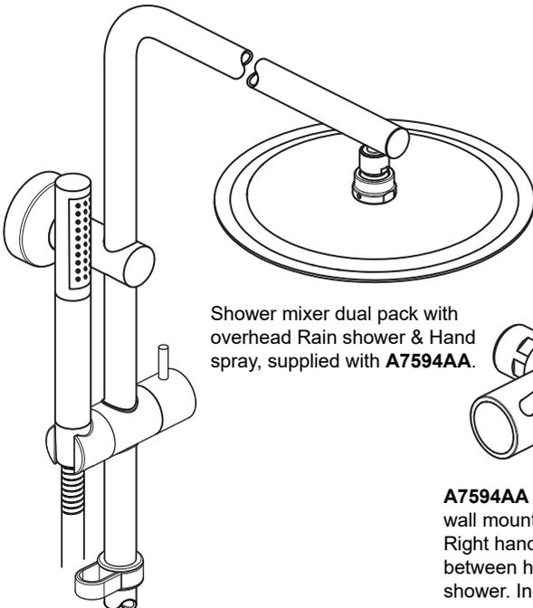
**A7594AA** Shower valve shown without wall mounting brackets assembled. Right handle controls flow & diverts between hand spray & overhead rain shower. Includes dual shower pack shown below.
