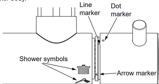
**IMPORTANT:** Before engaging the handle onto the diverter drive spindle, refit the plastic drive insert then: Align the dot marker on the handle with the line marker on the stop-sleeve. Reverse the sequence to refit the handle
