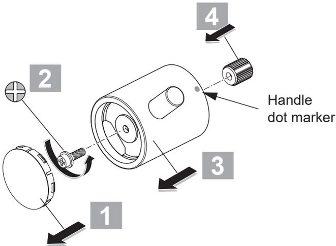
To gain access to either the thermostatic, flow or diverter cartridges, it will be necessary to remove the appropriate handle.
