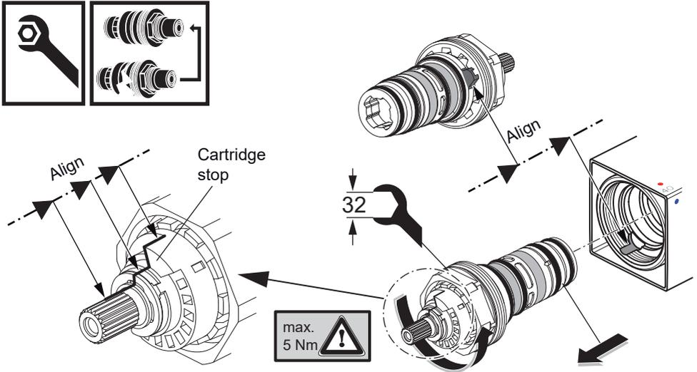
Use the following method to inspect or replace the thermostatic cartridge:
