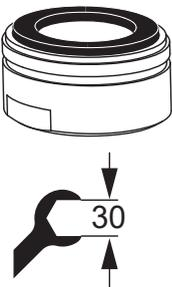
On a regular basis the anti-splash nozzle on the bath mixer should be inspected and cleaned if necessary
