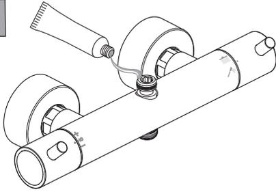
Note: the mixer supplied with A7594AA is fitted with an additional outlet nipple on the top surface to connect the over head shower plate.
