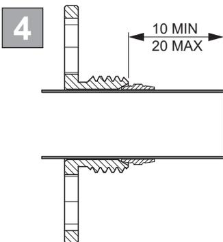
With the wall brackets in position, the supply pipes should be trimmed as shown. The pipes should project from the front face of the brackets by between 10 to 20mm.
