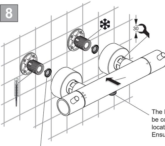
Assemble the shower mixer to the adaptors remembering to ensure that the sealing washers/ filters are inserted between the adaptors and the shower valve inlets. Keep the mixer parallel to the wall whilst screwing the captive nuts clockwise by hand. Carefully use a 30mm A/F spanner or strap wrench to tighten and make a water tight seal.
