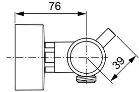
Basic bar shower mixer dimensions shown with wall mounting brackets assembled
