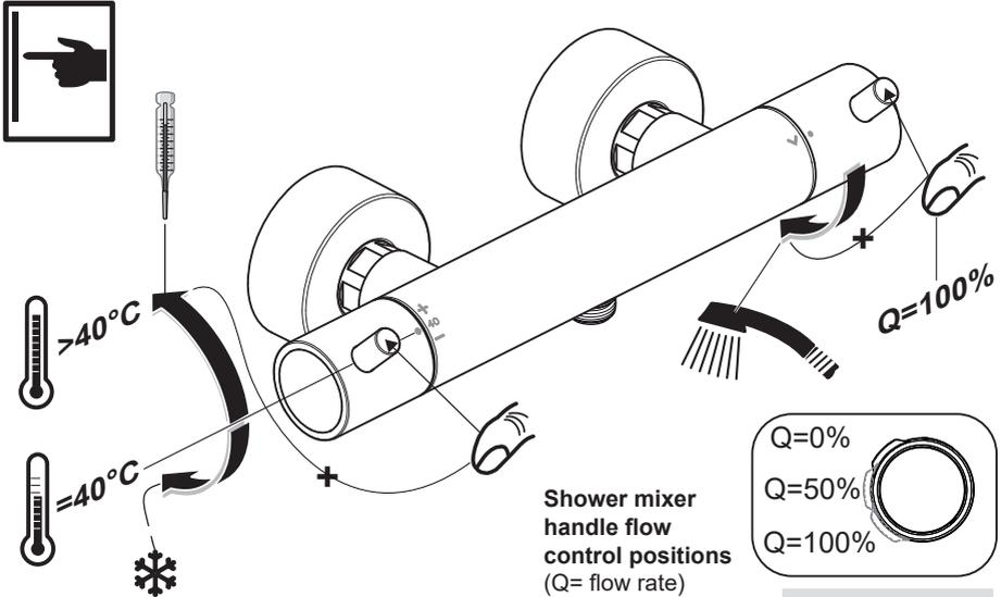
**NOTE:** the functionality of the temperature control handle is the same for all the products in the T125 range. A7592AA has a basic flow control handle, the other products have integral flow control & diverter for dual shower outlets/ bath fill.
