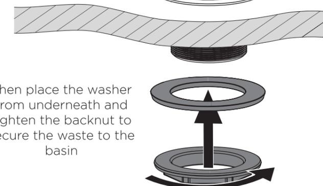
Then place the washer from underneath and tighten the backnut to secure the waste to the basin
