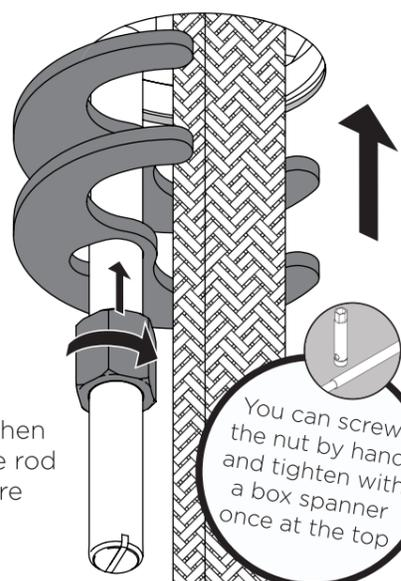
You can screw the nut by hand and tighten with a box spanner once at the top
