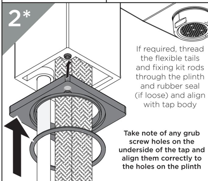
If required, thread the flexible tails and fixing kit rods through the plinth and rubber seal (if loose) and align with tap body
