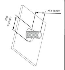
Install a ½" male threaded connection at the desired height on wall, ensuring that a minimum of 10mm of thread protrudes past the finished wall.
