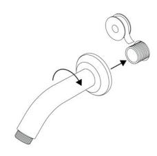
Apply plumbing tape to pipe. Screw arm onto pipe ensuring that the arm ends in the correct position.
