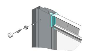
WHEN THE FRAME IS READY TO BE FIXED, DRILL THROUGH THE FRAME HOLES WITH A 3mm DRILL. (ENSURE YOU ONLY DRILL THROUGH ONE WALL THICKNESS OF THE WALL PROFILE). THEN FIX THE FRAME WITH ITEMS 19, 21 & 22
