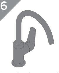
Turn on the mains water supply, letting the water flow for a few minutes to flush through the system.
