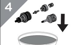
Remove any O-rings and soak all components in de-scaler and wash off in clean water. Examine all seals and replace if needed. Use WRAS approved silicon based grease on all seals.
