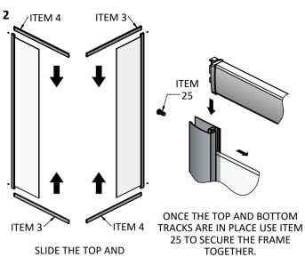
BOTTOM TRACKS; LH & RH, INTO THE GLASS PROFILES UNTIL FLUSH.
