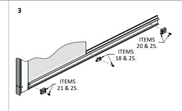
FIT THE BOTTOM GLASS CLIPS (ITEMS 18 & 19) UNDER THE GLASS. ONLY TIGHTEN SCREW PART WAY. FIT THE TOP GLASS CLIPS (ITEMS 18 & 19) AND TIGHTEN ALL SCREWS.
