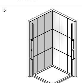
MAKE SURE THE WALL PROFILES ARE TRUE WITH A SPIRIT LEVEL. MARK THROUGH THE FIXING HOLES WITH A PENCIL. REMOVE PROFILES, DRILL AND PLUG THE WALL, (ITEM 27). THE WALL PLUGS SUPPLIED MAY NOT BE SUITABLE FOR YOUR SUBSTRATE, USE SUITABLE FIXINGS. NOW REFIT WALL PROFILES IN PLACE USING ITEM 22, 23 & 24.
