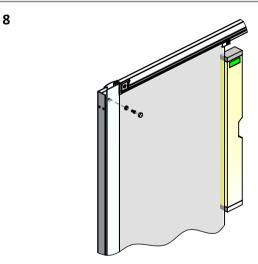
ENSURE SQUARE BEFORE FIXING. DRILL THROUGH THE HOLES IN THE FIXED GLASS PANEL PROFILES WITH A 3mm DRILL BIT.
