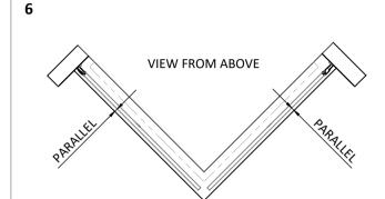
FIT THE FRAME OVER THE WALL PROFILES, ADJUST SO THE GLASS IS PARALLEL TO THE TRAY EDGE. THERE SHOULD ALSO BE AN EQUAL AMOUNT OF FRAME IN EACH WALL PROFILE. ENSURE THE FRAME IS TRUE AND SQUARE ON BOTH SIDES BEFORE FIXING THE TWO FRAMES TOGETHER, USE A SPIRIT LEVEL ON THE EDGE OF THE FIXED GLASS PANEL.
