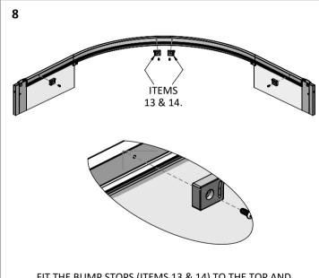
FIT THE BUMP STOPS (ITEMS 13 & 14) TO THE TOP AND BOTTOM TRACKS WITH ITEM 21. DO NOT OVERTIGHTEN THE SCREW, OTHERWISE IT WILL SHOW THROUGH ON THE FRONT FACE OF THE TRACK.
