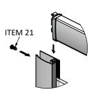
ONCE THE TOP & BOTTOM TRACKS ARE IN PLACE USE ITEM 21 TO SECURE THE FRAME TOGETHER.
