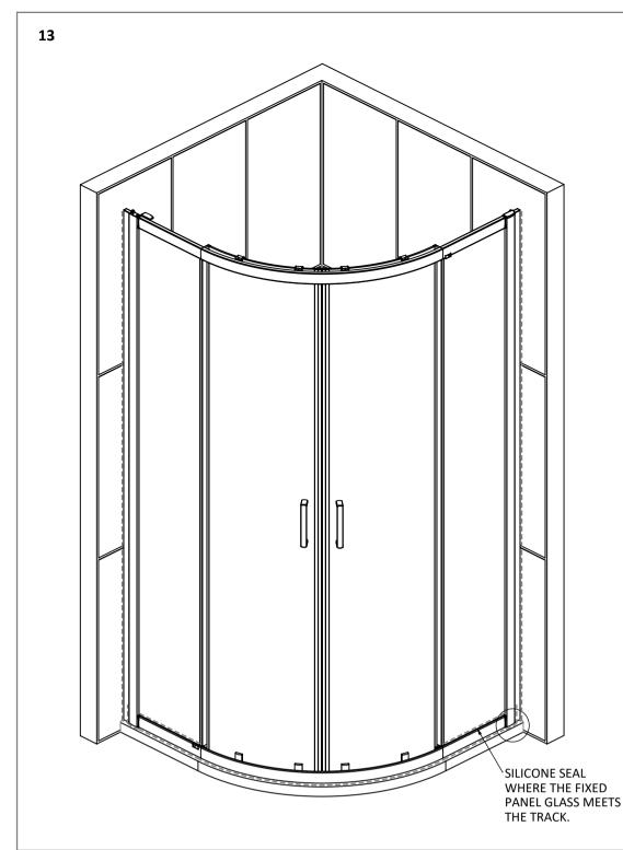
EXTERNALLY SILICONE SEAL THE WALL PROFILES WHERE THEY MEET THE WALL AND THE BOTTOM PROFILE WHERE IT MEETS THE TRAY. ALL IN A CONTINUOUS BEAD.
