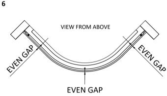
FIT THE FRAME OVER THE WALL PROFILES, ADJUSTING UNTIL THERE'S AN EVEN GAP BETWEEN THE FRONT EDGE OF THE TRAY AND BOTTOM TRACK. THERE SHOULD ALSO BE AN EQUAL AMOUNT OF FRAME IN EACH WALL PROFILE. ENSURE THE FRAME IS TRUE AND SQUARE ON BOTH SIDES BEFORE IT IS FIXED IN PLACE, USE A SPIRIT LEVEL ON THE EDGE OF THE FIXED GLASS PANEL.
