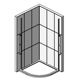
MAKE SURE THE WALL PROFILES ARE TRUE WITH A SPIRIT LEVEL. MARK THROUGH THE FIXING HOLES WITH A PENCIL. REMOVE PROFILES, DRILL AND PLUG THE WALLS (ITEMS 22). THE WALL PLUGS SUPPLIED MAY NOT BE SUITABLE FOR YOUR SUBSTRATE, USE SUITABLE FIXINGS. FIX THE WALL PROFILES IN PLACE USING ITEM 20.
