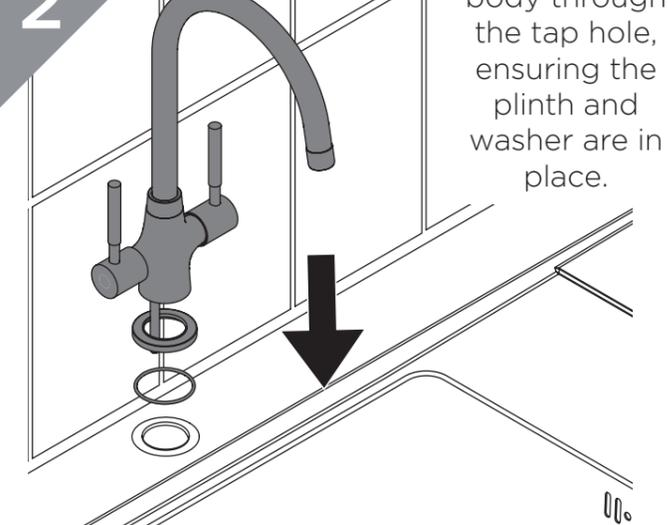
Feed the tap body through the tap hole, ensuring the plinth and washer are in place.
