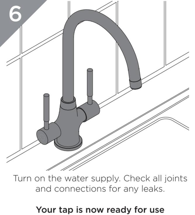
Turn on the water supply. Check all joints and connections for any leaks.
