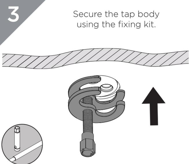
Secure the tap body using the fixing kit.
