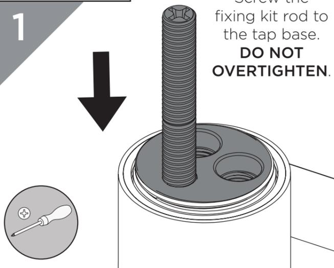
Screw the fixing kit rod to the tap base.
