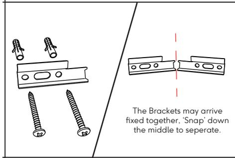
The Brackets may arrive fixed together, 'Snap' down the middle to separate.
