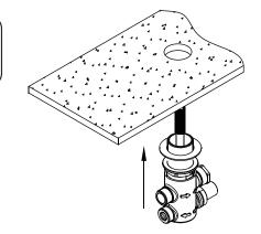
Connect the handle set tightly with the bottom valve kit
