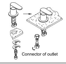
Take out the diverter valve set, disassemble the handle set
