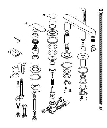
Prepare the cartridge set ,disassemble the bottom installation kit
