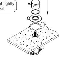
Using spanner to fix on the fixing screw in clockwise rotation and put on the plug
