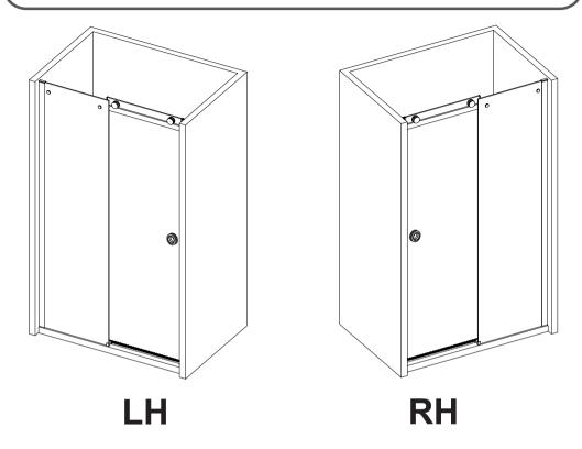
The slider is ok to be installed in left hand and right hand. The following step is based on left hand. For right hand, please follow the step in mirror direction.
