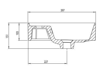
Diagrams not to scale All dimensions in mm tolerance of +/-5mm
