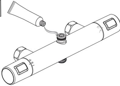
Note: the mixer supplied with A7209AA is fitted with an additional outlet nipple on the top surface to connect the over head shower plate.
