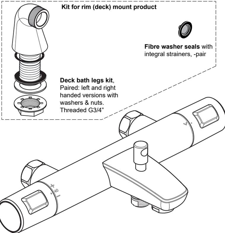
Deck bath/shower mixer shown without deck mounting legs assembled. Supplied with both **A7207AA & A7698AA** product. Right side handle controls flow. Diverter operates through the spout. Note: **A7207AA** is supplied without a shower kit, & **A7698AA** with supplied with the 600 riser rail & handset pack.
