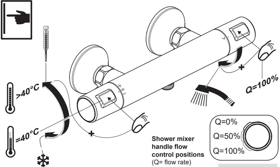
**NOTE:** the functionality of the temperature control handle is the same for all the products in the T25 range. A7209AA has a basic flow control handle, the other products have integral flow control & diverter for dual shower outlets/ bath fill.
