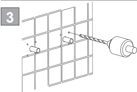
Drill holes appropriate for your choice of fixings into the wall.
