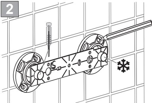
Place the brackets over the exposed pipes and use the template provided to position them 150mm apart.
