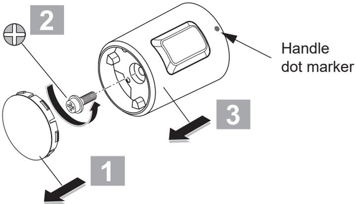
To gain access to either the thermostatic, flow or diverter cartridges, it will be necessary to remove the appropriate handle.
