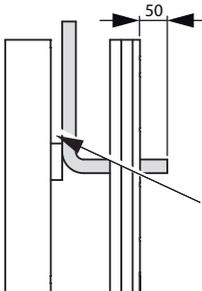
We recommend leaving 50mm of pipe protruding at this stage.
