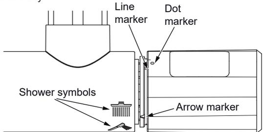
**IMPORTANT:** Before engaging the handle onto the diverter drive spindle, refit the plastic drive insert then: Align the dot marker on the handle with the line marker on the stop-sleeve. Reverse the sequence to refit the handle
