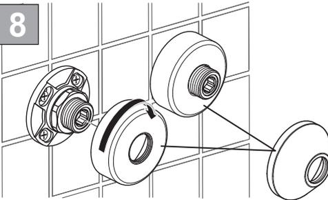
When the sealant has set, fit the covers by screwing them onto the adaptors until they are flush with the wall.
