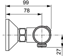
Basic bar shower mixer dimensions shown with wall mounting brackets assembled
