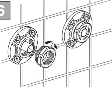
Screw the brass adaptors over the pipes into the plastic brackets. 36mm A/F Spanner flats are provided, hand tightness is adequate.
