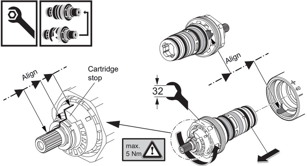
Use the following method to inspect or replace the thermostatic cartridge:
