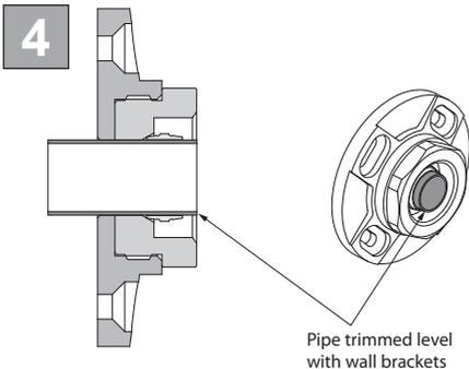
The pipes should be trimmed level to the wall bracket. If using a pipe cutter it will be necessary to mark the pipes and then remove the bracket before trimming to its correct length.
