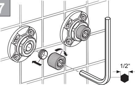
Fit the olives to the pipes prior to screwing the two 3/4" connectors into the wall mount plate using a 1/2" allen key. The connectors will have to be securely screwed in to form the necessary compression joint between the olive, wall plate and connector. Retain the brass adaptors with a spanner when making the compression joints.
