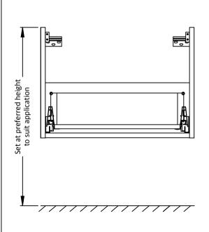
Fix Wall Hanging Plates as shown above. Check the type of wall you are fixing into and use suitable fixings (Not supplied).
