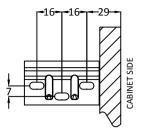
You may need to lengthen the hook's protrusion. To do so, turn screw 'B' anti-clockwise.
