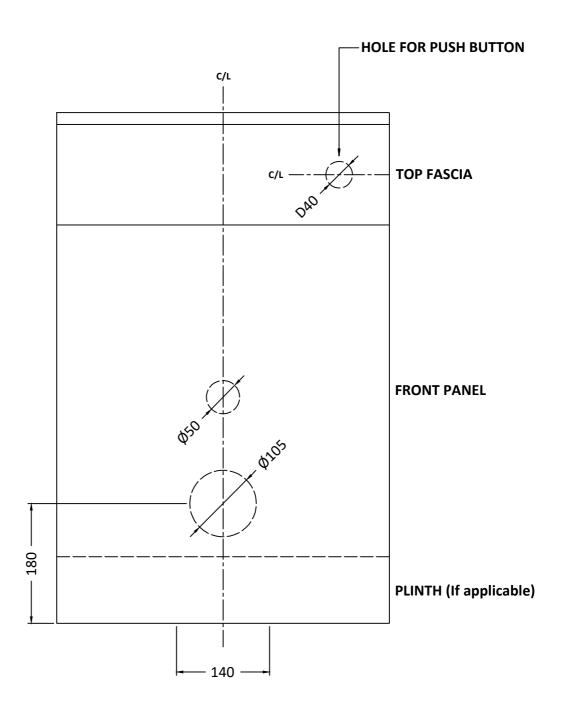
MARK OUT THE HOLE POSITIONS ON THE FRONT PANEL FOR THE INLET AND OUTLETS OF THE W.C. PAN. CHECK THE SIZE AGAINST THE PAN BEFORE CUTTING OUT. DO NOT CUT FULLY THROUGH THE BOTTOM PLINTH!
