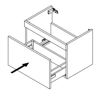
To re-fit the drawer, fully extend the drawer runners and locate drawer box on to runners. Push the drawer box fully home until you here a 'click'. The drawer drawer should now be correctly located onto the runners.
