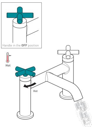
Turning the hot handle to the left will increase the flow of hot water.
