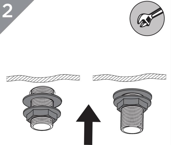
Secure the taps to the basin by using the washer and metal backnut below the basin.
