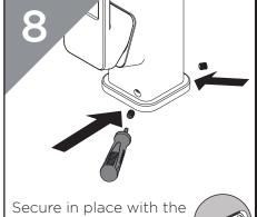
grub screws using the tool provided.
