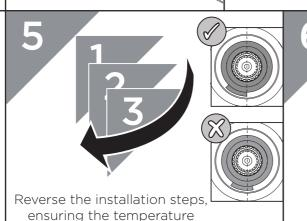
stop is aligned correctly.
