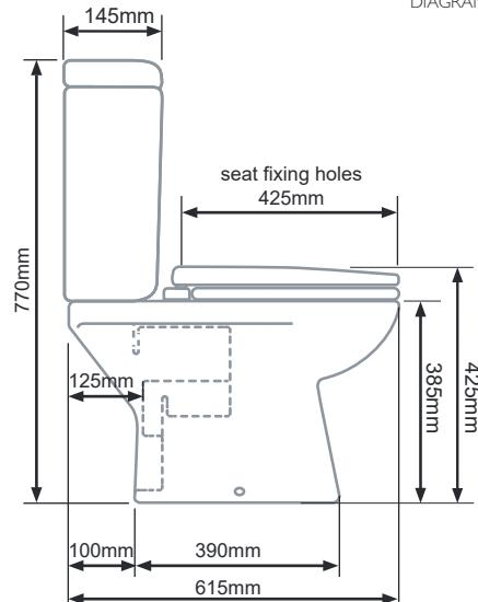
DIAGRAMS NOT TO SCALE | ALL DIMENSIONS IN MM TOLERANCE OF  $\pm 5\text{MM}$
