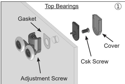
1. Carefully dismantle the Bearing Assemblies, place the gasket on the outside of the glass (Bearing Side) then re-assemble onto the Door Glass. Make sure you have the correct bearings at the top and bottom and that the wheels are on the outside of the glass.
