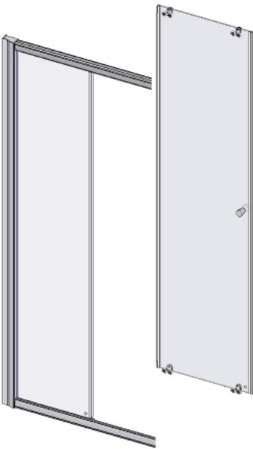
1. Carefully lift the assembled doors into the enclosure ensuring that it is the correct way round.
