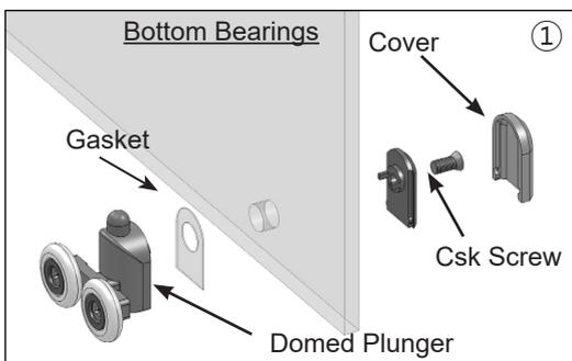
**NOTE: The Bearing Assemblies for the top and bottom are different and can be distinguished by the bottom bearings having a domed plunger.**
