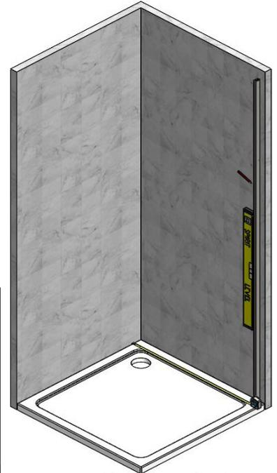
\*Only one profile shown here - both profiles are fitted at this stage.
