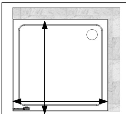
Measure from the very outside of the tray - before the radius. Go all the way to the tiled wall.
