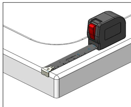
Measure from the very outside of the tray - before the radius. Go all the way to the tiled wall.
